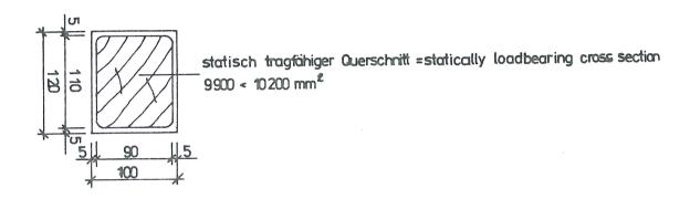
Thus, a protective layer of timber amounting to 5 mm is remaining as a structural corrosion protection.
